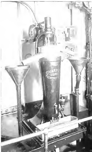
The Sharples super centrifuge as installed for cleaning the lubricating oil on the Matson liner Maui.
